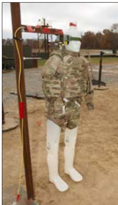
This mannequin is outfitted with soft armor components and hard armor plates for blast testing.
