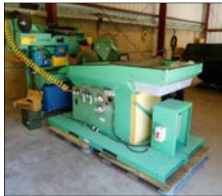
Down-draft table at head end of SBS system.
