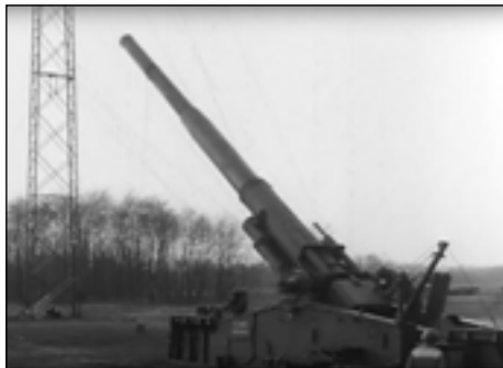
The 280mm Atomic Cannon test firing an inert W9 atomic artillery projectile at APG
